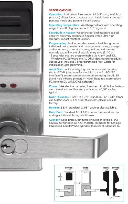
core models accept Arrow®, Best®. Falcon®, KSP® and Kaba Peaks® 6 or 7 pin IC core cylinders (not furnished). Alarm Lock tailpiece for use with IC core cylinders is furnished. IC core models prepped for Yale®, Medeco®, Corbin-Russwin®, Sargent® and Schlage® also available.
